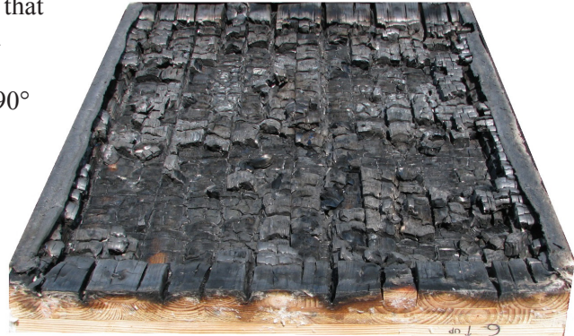
CLT specimen exposed to the standard time–temperature curve from ASTM E 119.
