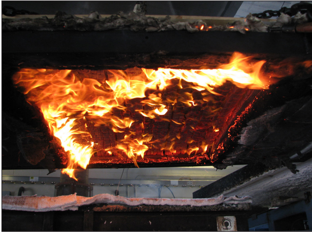
CLT specimen being removed from furnace.
