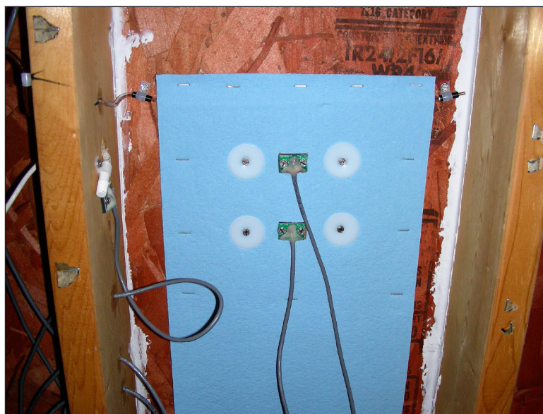
Figure 9. Water injection system.
