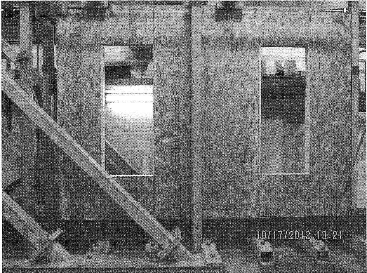
Figure 7. Cyclic Load Test Machine with Test 2A Wall (Test 2B Similar) in Place.
