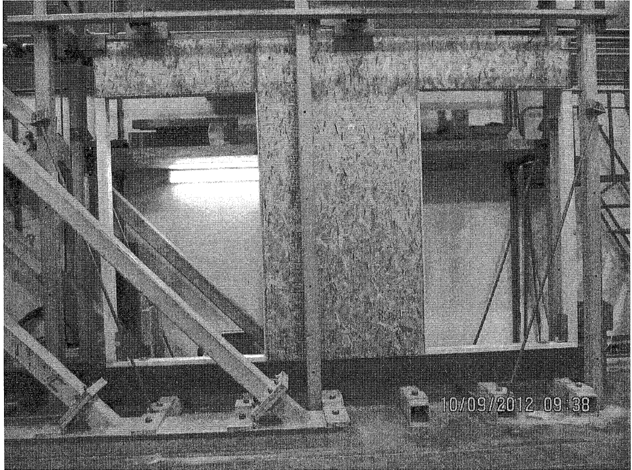
Figure 3. Cyclic Load Test Machine with Test C-1 (Control) Wall in Place.
